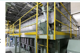
"KG-18-T" hydrogen Mixed-fuel Large Gas Engine
