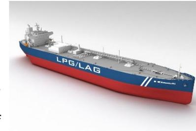
Image of LPG/LAG carriers of 86,700m<sup>3</sup> class by LPG fuel
