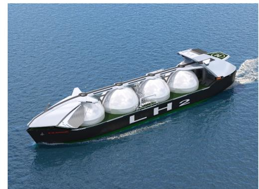
Image of large liquefied hydrogen carrier
