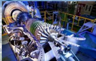
Hydrogen gas turbine
