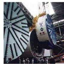
Excavation on the Tokyo Bay Aqua-line completed by world's largest shield machines.
