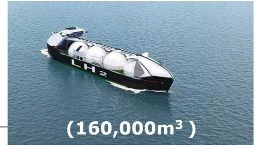
By upscaling the ships, the volume transported will increase by **128 times** (however, the construction cost will increase by several times)
