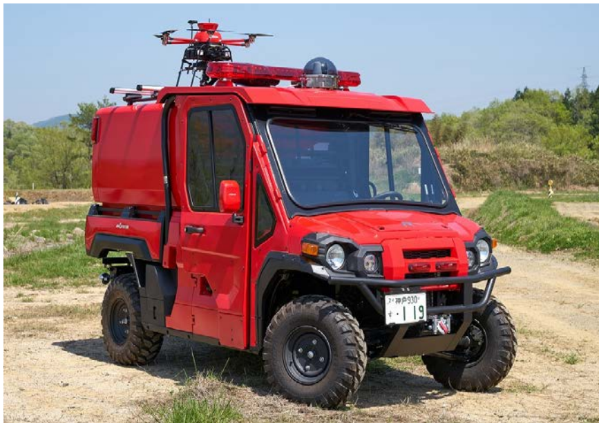
Compact size off-road fire-fighting vehicle “Red Ladybug” (Developed based on Kawasaki MULE PRO-FX EPS)
