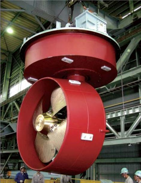
Azimuth thruster Rexpeller®
