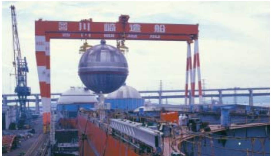
Two 800t Goliath cranes can lift and put into place an entire LNG tank
