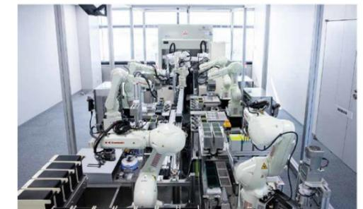
Automated robotic PCR testing system
