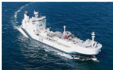
Suiso Frontier liquefied hydrogen carrier
