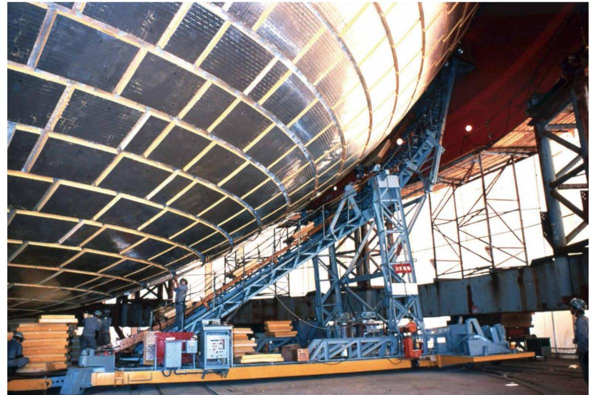
Construction of Kawasaki Panel System, Kawasaki's proprietary insulation system for LNG carrier tanks
