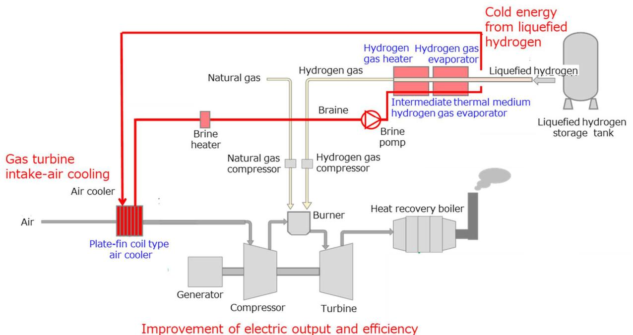
Structure of a gas turbine intake-air cooling system that utilizes cold energy from liquefied hydrogen
