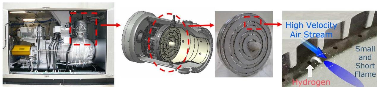
Gas turbine unit and dry low NO<sub>x</sub> combustor using micro-mix combustion technology
