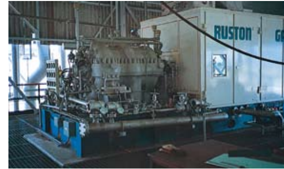
Gas turbine driven compressor for HC mixt. gas service, PERTAMINA (Indonesia)
