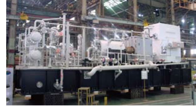
Motor driven compressor for natural gas service, ZADCO (UAE)
