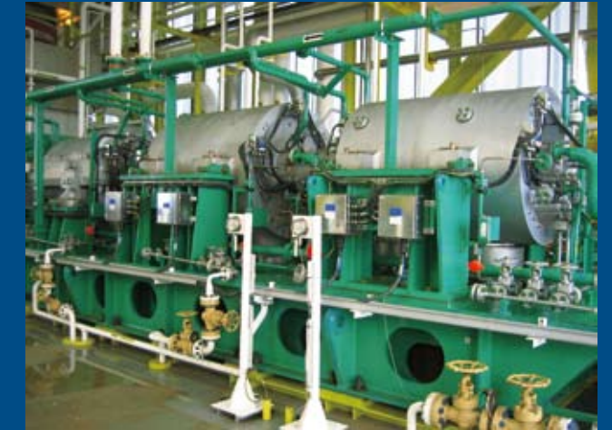
Triple tandem arranged gas turbine driven compressors, PSCB (Malaysia)
