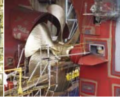
Kawasaki's proprietary semi-duct system with contra fins and rudder bulb with fins enhance propeller efficiency.
