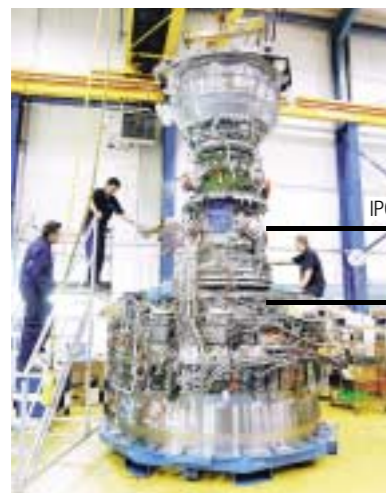
This is the location of the IPC module in the Trent 1000. Photo taken at Rolls-Royce's Derby plant.
