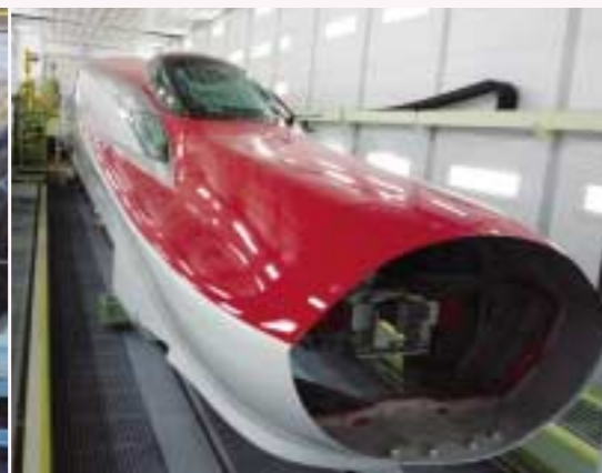
The front car is painted and dried at Kawasaki's new paint facility inside the Hyogo Works, which was completed in December 2009.
