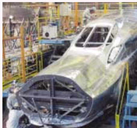
Manufacturing the front car. The aerodynamic curves of the car's elongated nose are mostly crafted by hand.
