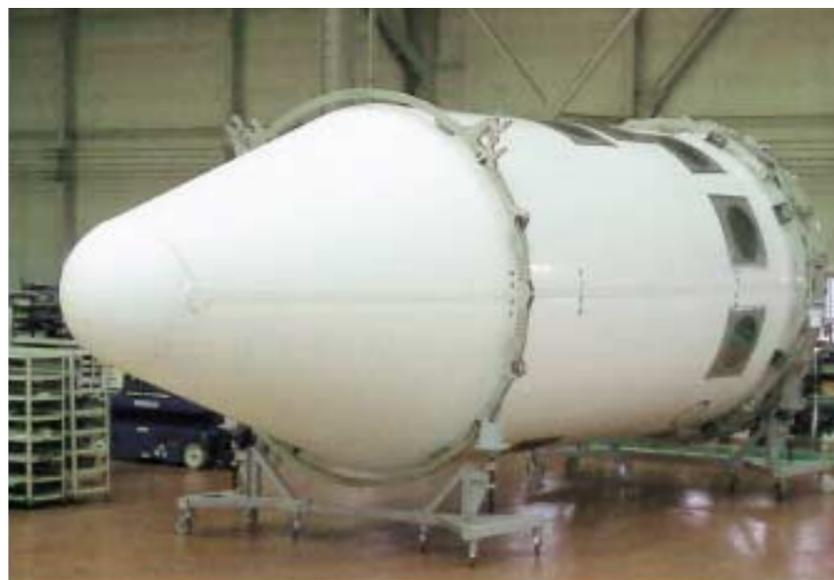
This past June Kawasaki delivered the payload fairing for the Japan Aerospace Exploration Agency (JAXA) H-IIA Launch Vehicle No.13 (H-IIA F13) to the Tanegashima Space Center. The launch of the H-IIA F13 was conducted on September 14, 2007. The payload fairing is
