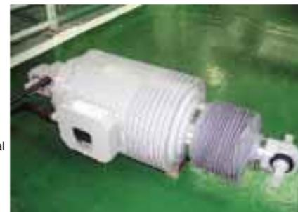
An actuator for the active suspension system
