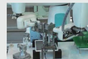
Inspection of functions and response capabilities of a touch screen
