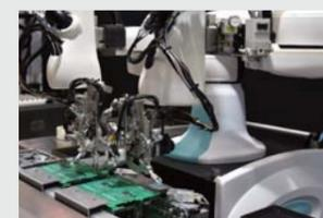
Mounting of parts on a PCB
