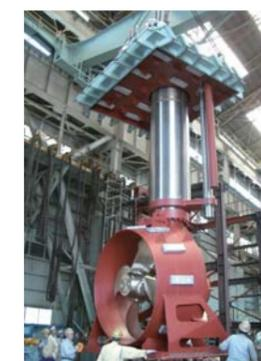
The retractable Rexpeller can be retracted into the hull by hydraulic means, allowing the vessel to sail at high speed by reducing hull resistance during transportation.
