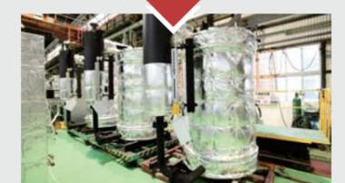
The boiler is then fitted with sensors and "clothed" with insulation sheets. This is the semi-final stage of boiler construction.
