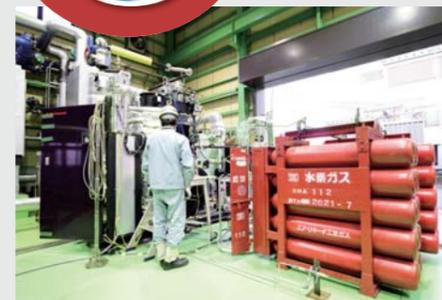
A hydrogen-fired once-through boiler used for the verification testing. The red tank contains the hydrogen.
