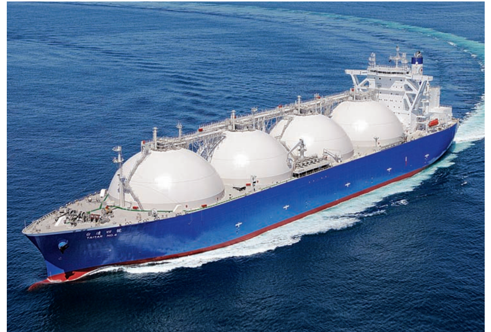
TAITAR NO.4 Length/289.50m Breadth/49.00m Depth/27.00m Draft/11.90m Tank capacity/147,546m 3 DWT/77,053t Delivery/2010
