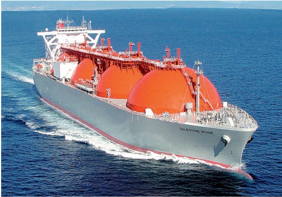
CELESTINE RIVER Length/289.70m Breadth/49.00m Depth/27.00m Draft/11.40m Tank capacity/147,608m 3 DWT/71,646t Delivery/2007
