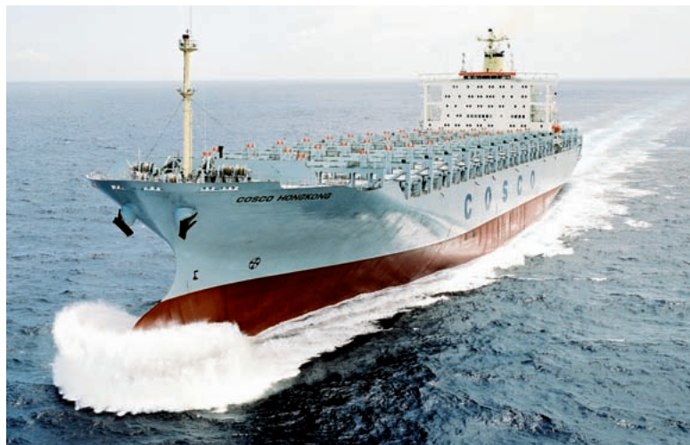
COSCO HONGKONG Length/280.00m Breadth/39.80m Depth/23.60m Draft/14.00m DWT/69,207t Container capacity/5250TEU Delivery/2002
