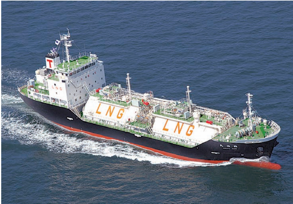
鶴佑丸 KAKUYUMARU Length/88.80m Breadth/15.30m Depth/7.20m Draft/4.30m Tank capacity/2,538m 3 DWT/1,865t Delivery/2013
