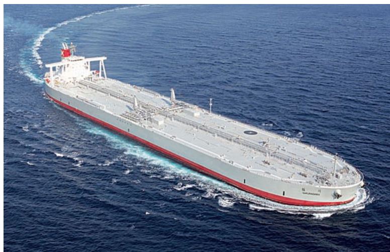
SAKURAGAWA Length/332.93m Breadth/60.00m Depth/29.00m Draft/20.305m DWT/299,982t Delivery/2009
