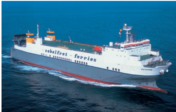
VICTORINE Length/162.49m Breadth/25.20m Depth/15.45m Draft/6.50m Car capacity/trailer155+automobile 446 DWT/9,729t Delivery/2000
