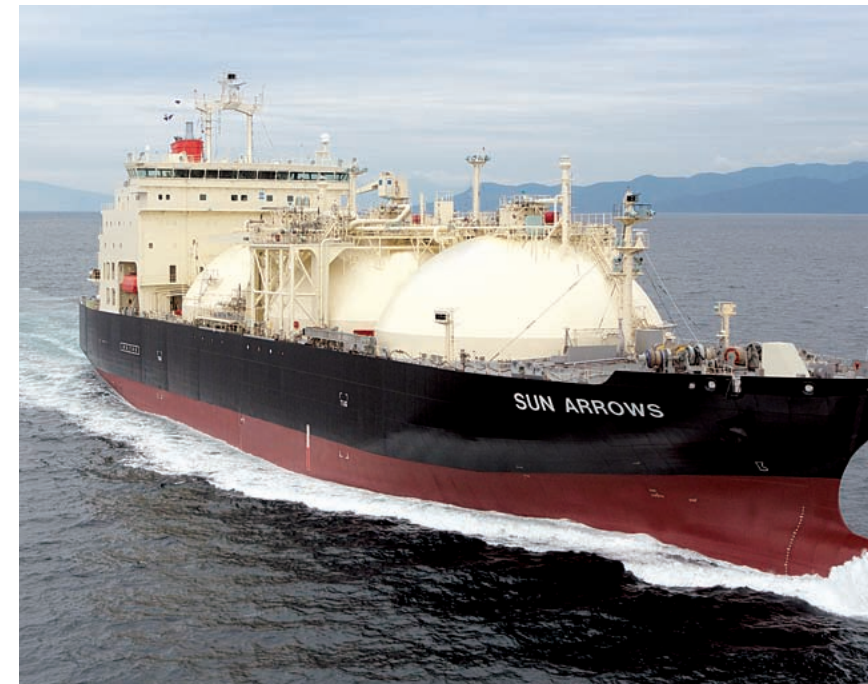
SUN ARROWS Length/151.00m Breadth/28.00m Depth/16.00m Draft/7.30m Tank capacity/19,468m³ DWT/10,130t Delivery/2007
