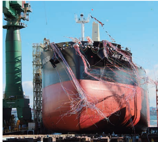
AMIS GLORY Length/189.90m Breadth/32.26m Depth/17.90m Draft/12.50m DWT/55,000t Delivery/2016
