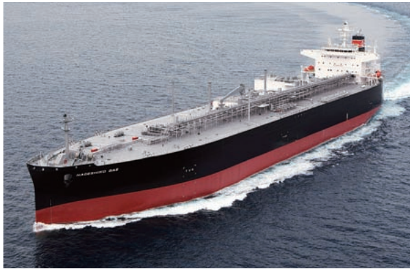
NADESHIKO GAS Length/226.00m Breadth/37.20m Depth/21.00m Draft/11.20m Tank capacity/80,152m 3 DWT/53,003t Delivery/2013
