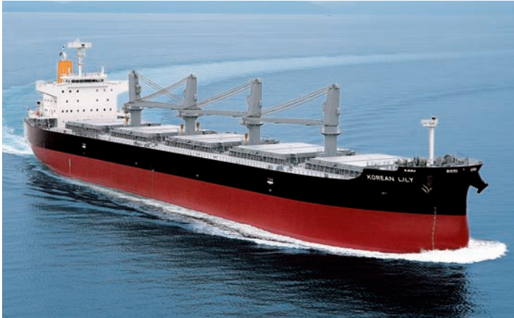
KOREAN LILY Length/197.00m Breadth/32.26m Depth/18.10m Draft/12.65m DWT/58,713t Delivery/2010
