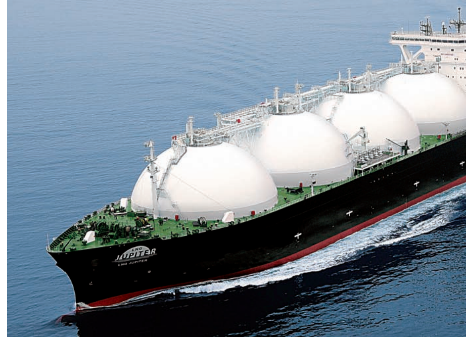
LNG JUPITER Length/289.50m Breadth/49.00m Depth/27.00m Draft/11.90m Tank capacity/155,999m³ DWT/76,355t Delivery/2009
