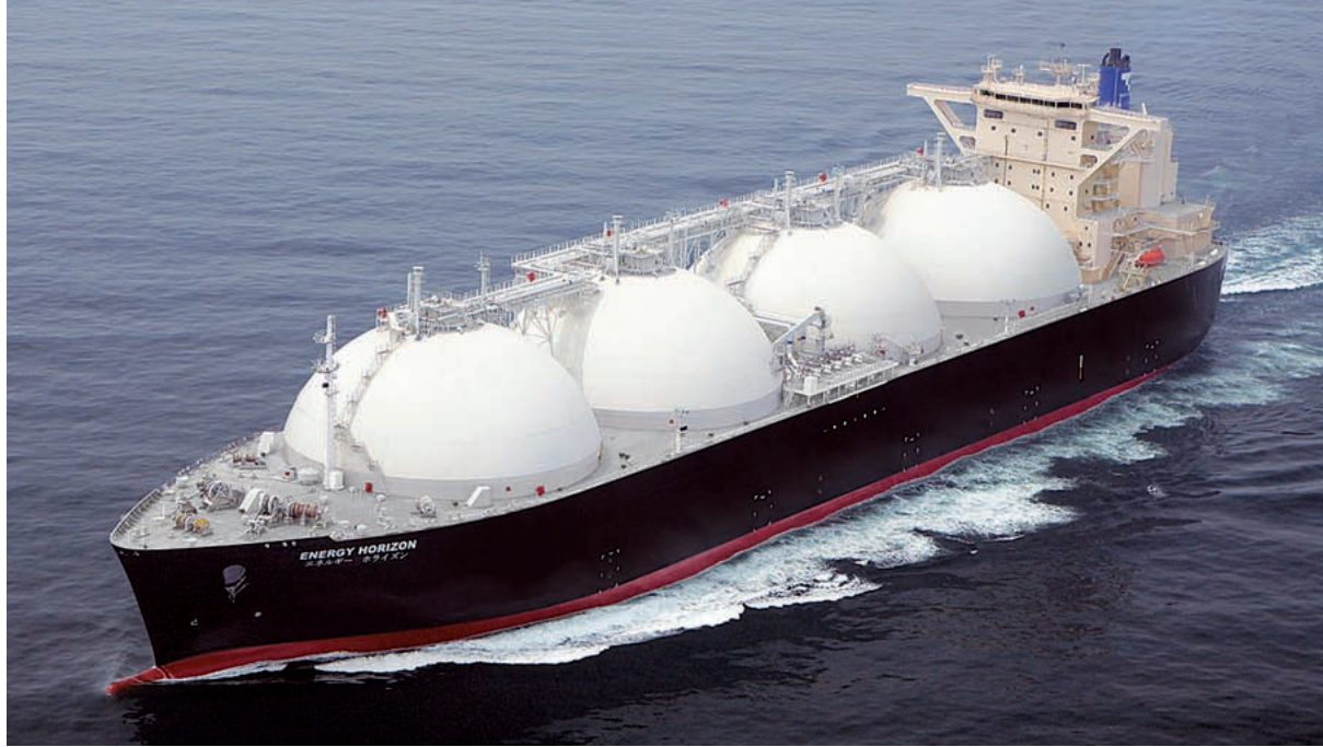
ENERGY HORIZON Length/300.00m Breadth/52.00m Depth/28.00m Draft/11.65m Tank capacity/177,440m³ DWT/87,257t Delivery/2011
