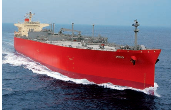
HISUI Length/226.00m Breadth/37.20m Depth/21.00m Draft/11.20m Tank capacity/80,199m 3 DWT/53,012t Delivery/2010
