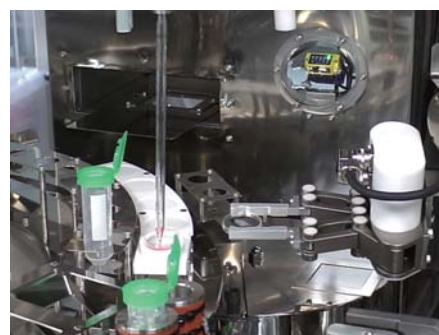
Manipulation of various vessels including dishes using a multi-purpose hand
