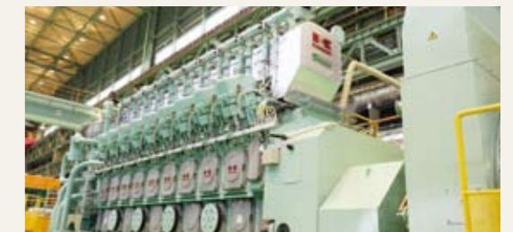
The Green Gas Engine boasts the world's highest power generating efficiency—49.5%.
