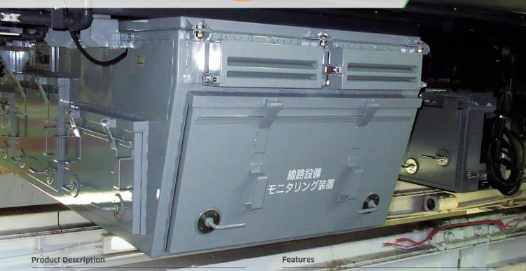
A device equipped to the underfloor space of trains in commercial operation to obtain the image data of track materials (rails, rail fasteners and fish bolts) using laser beams, while traveling at up to 130 km/h in order to check for missing or loose bolts.  Compact design enables the device to be equipped to the underfloor space of trains in commercial operation
