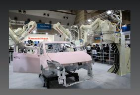
• Offers space-saving advantages, thanks to integrated treatment of painting cables inside the
