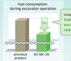
Using the latest control technology, fuel consumption during excavator operation was reduced by 15%.
