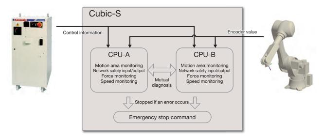
Fig. 1 Basic configuration of Cubic-S
