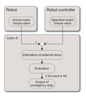
Fig. 3 Process flow of force monitoring function
