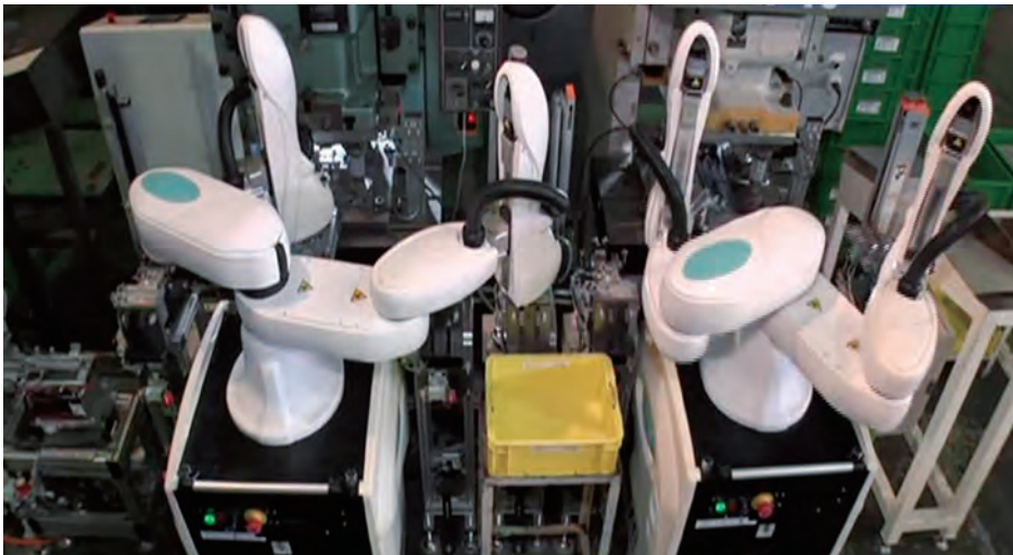
Fig. 7 Application of loading/unloading for pressing machine
