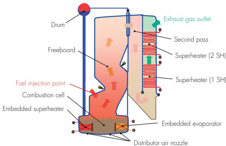
Fig. 2 Overall view of internal circulation fluidized bed boiler
