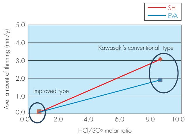
Fig. 9 Comparison between HCl/SO<sub>2</sub> gas ratio and annual embedded tube corrosion amount
