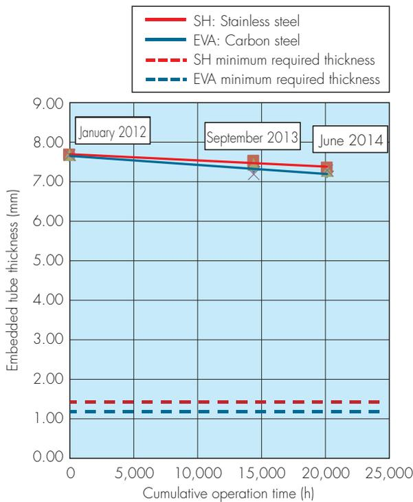
Fig. 8 Cumulative operating time and embedded tube thinning in internal circulation fluidized bed boiler for South Korea
