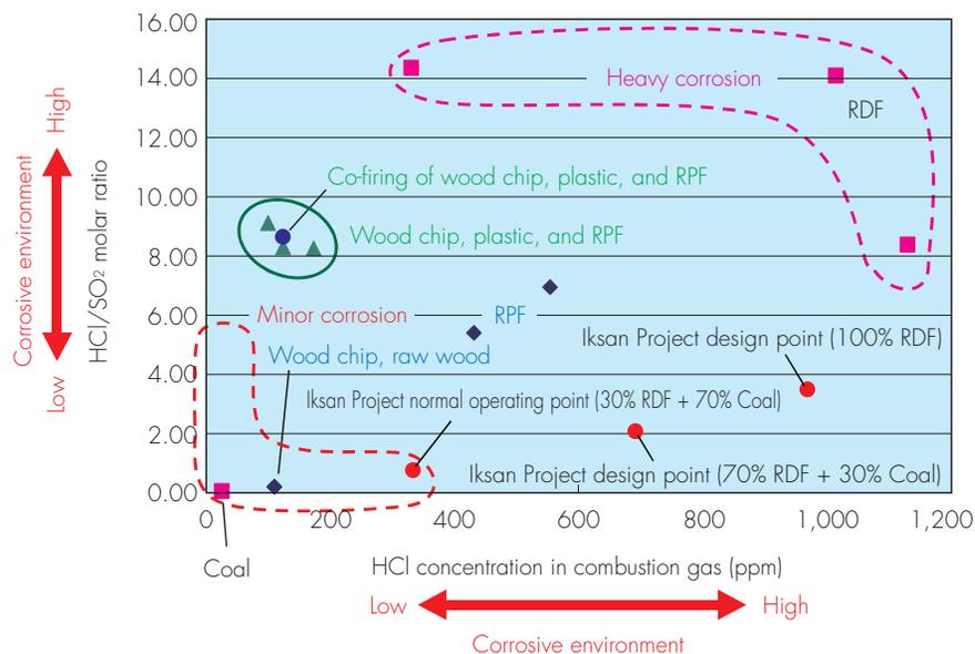
Fig. 7 Impact of HCl/SO<sub>2</sub> ratio in combustion gas on corrosion
