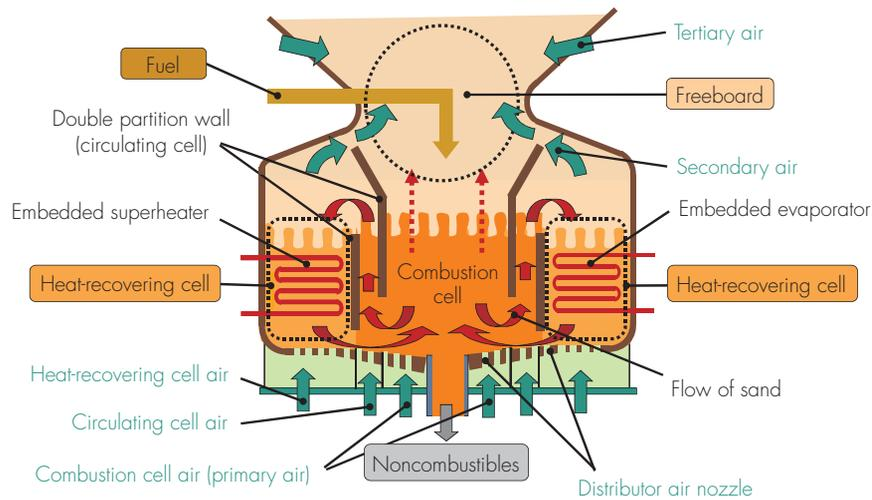
Fig. 1 Conceptual diagram of internal circulation fluidized bed boiler
