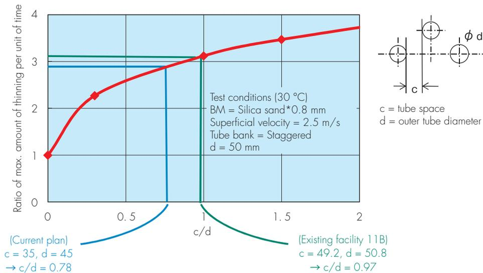
Fig. 6 Relationship between horizontal pitch of embedded tubes and thinning due to abrasion
