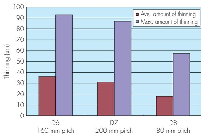
Fig. 5 Relationship between furnace width pitch of embedded tubes and tube wall thinning
