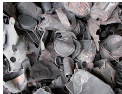
(b) Material recycled with magnetic separator
