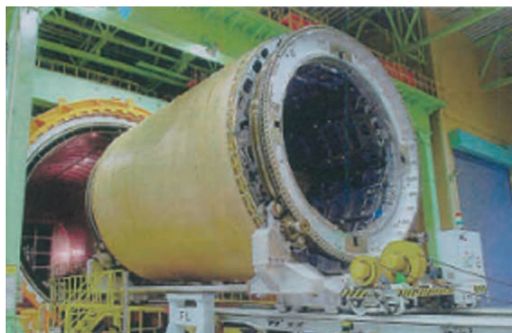
Fig. 3 Forward fuselage cured in an autoclave
