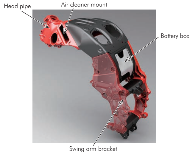
Fig. 10 Modified components of the aluminum monocoque frame
