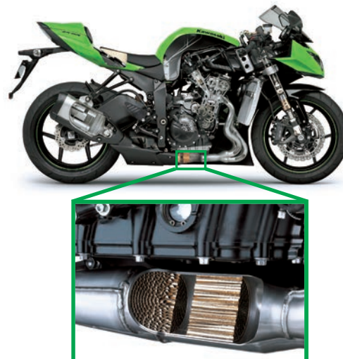
Fig. 8 Three-way catalyst for motorcycle (Honeycomb form)
