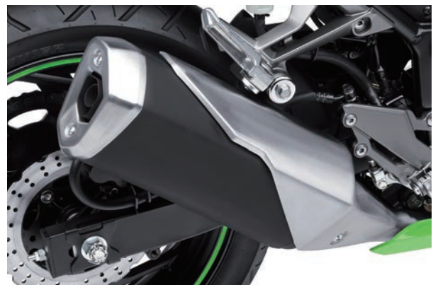
Fig. 7 Short muffler with complex cross-section
