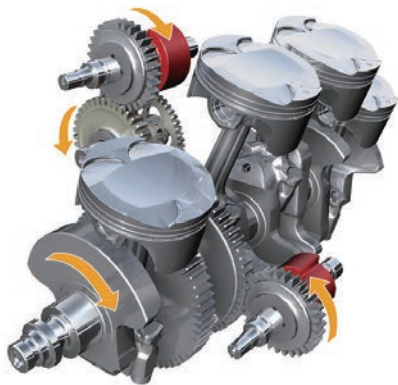
(a) Dual-shaft secondary balancers
