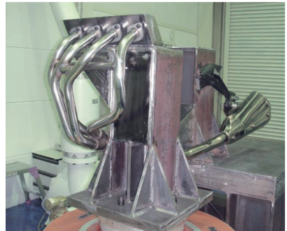
Fig. 7 Vibration test for exhaust system
