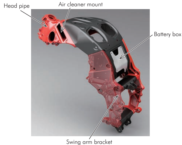
Fig. 10 Modified components of the aluminum monocoque frame
