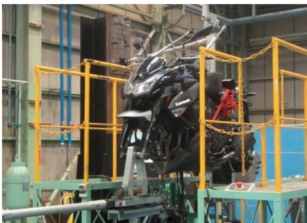
Fig. 12 Durability test using road simulator
