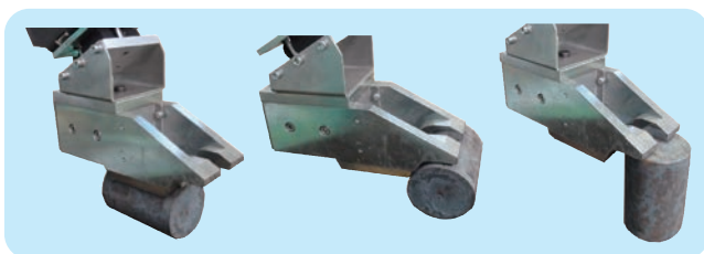
(a) Normal grip (b) Front edge grip (c) Bottom surface grip
