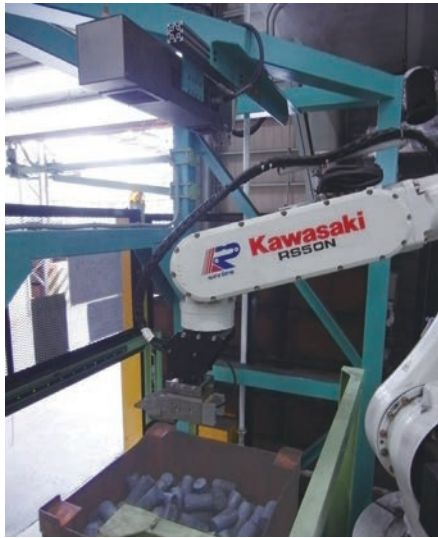
Fig. 9 Bin-picking system for forged part
