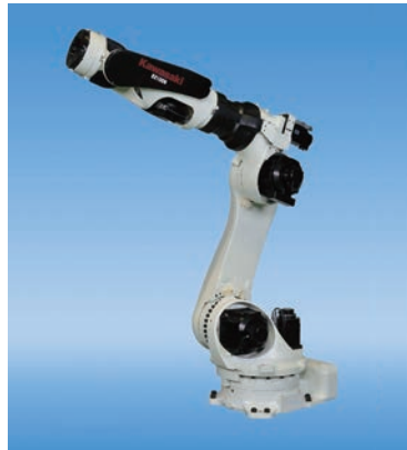
Wiring and piping housed in the hollow section at the center of the rotation axis
