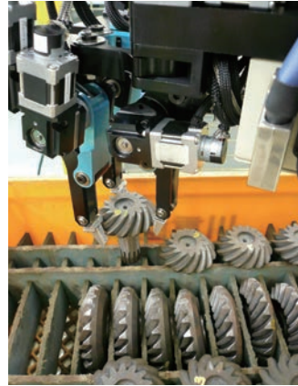
Fig. 2 Earlier version of the humanoid hand (2007)
