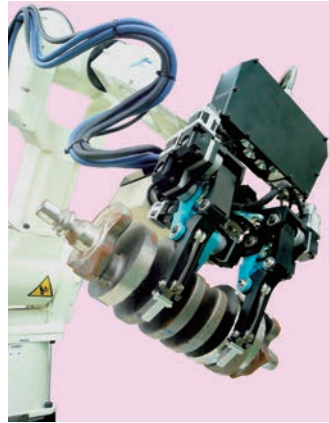
Fig. 2 Earlier version of the humanoid hand (2007)
