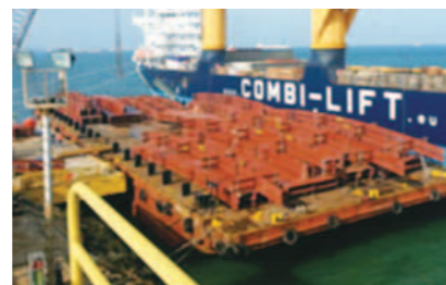
Shipment of LNG tank roof components made by Indonesian vendor is loaded for journey to project site in Australia
