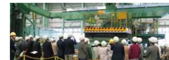
Watching an autoriveter at work on Boeing 777 panels
